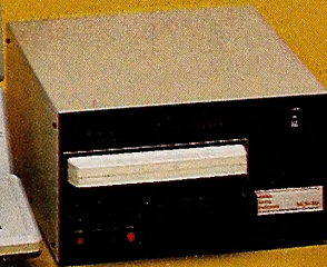
Shown below: Removable 8" 10 MByte Winchester cartridge drive.
